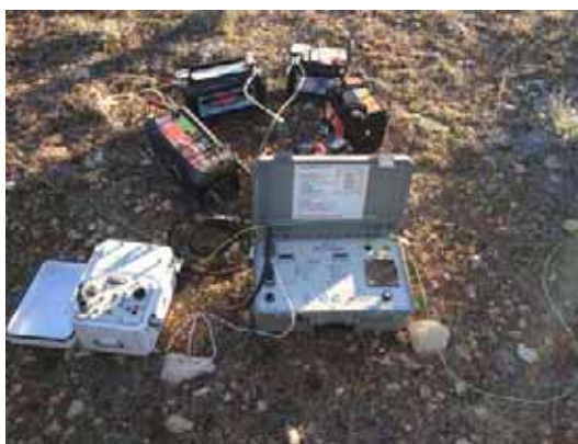
Figura 1.- Transmisor ZT-30 de Zonge Engineering and Research Organization.
