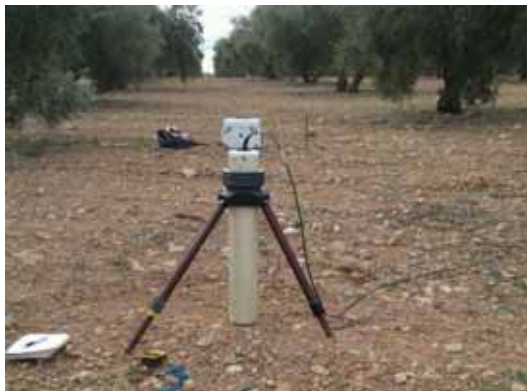
Figura 2.- Receptor GDP-32 II y antena TEM-3 de Zonge Engineering and Research Organization.
